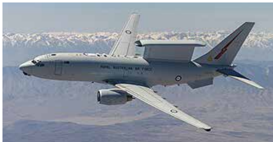
RAAF E-7A Wedgetail early Warning & Control Aircraft. Note the 'top-hat' on the dorsal fin housing the sophisticated radar giving the plane its distinctive profile.
